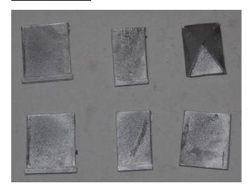
Assemble the front, back and two sides to form a box, with the sides inside the front and back. The beading should be on the outside and line up around the top.
