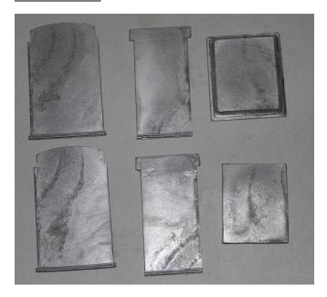
Assemble the front, back and two sides to form a box, with the sides inside the front and back and the extension pieces in the gaps of the front and back. The beading should be on the outside and line up at the bottom.
