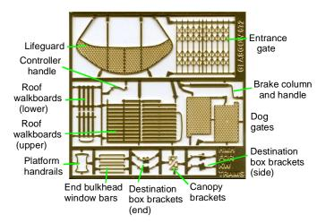
Carefully rub over all parts with fine sandpaper before removing from etch, to provide a key for glue/solder/paint. Rub along, rather than across, long narrow items as far as possible.
