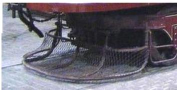
**Lifeguard:** Note that top front of lifeguard is sloped, not vertical. Bend mesh area horizontally to this angle, by rolling against a ruler with a needle file handle or similar, then work with fingers and thumbs to apply a curve in plan view to the sides and adjust overall shape. Bend hanging strips to vertical.
