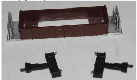
10. Cut the back off the truck sides if required to fit around the motor. Fix the truck sides and steps.
