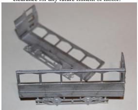
3. Assemble body sides and bulkheads into a box assembly, if necessary, removing excess beading to get a flush fit.
