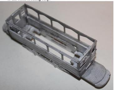
5. Now carefully bend the dash panels with lip on the upper edge to the shape of the platform, cut to length and fit to the platform.
