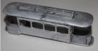
7. Carefully bend the vestibules to the shape of the dash panel and roof fit to the front of the dash panel and lower edge of the roof.
