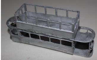
10. Trim the upper platform ends and carefully bend to shape and fit.
