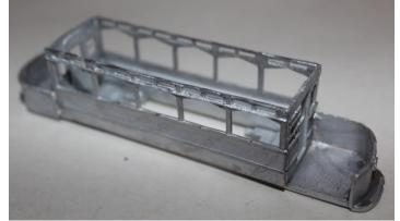
4. Fix the two halves of the ceiling/floor together and fit to the lower deck
