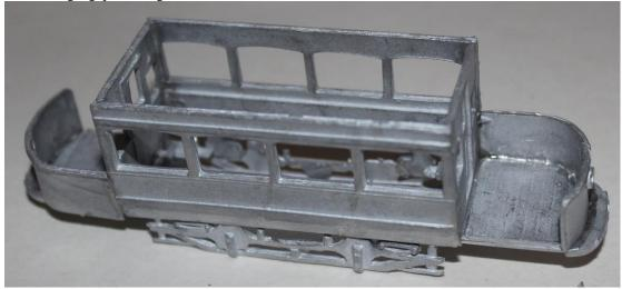
Fix the ceiling/upper deck floor piece Attach upper deck sides and ends to the floor.
