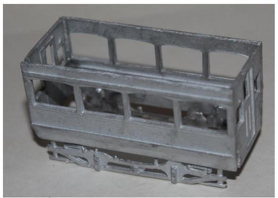
With model inverted, attach platforms to bottom edges of bulkheads; ensuring the lip is within the body and not on the platform.
