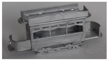
Turn model over and fit the steps and the life trays attached to the front edge of the truck sides so they do not interfere with the mechanism.
