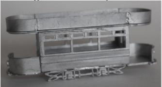
7. Turn model over and fix the life guards under the front panels and the life trays attached to the front edge of the truck sides so they do not interfere with the mechanism.
