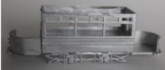
5. Fix the ceiling/upper deck floor piece
