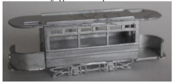
6. Attach upper deck sides and carefully bend the ends and trim to fit.
