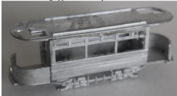
6. Attach upper deck sides and carefully bend the ends and trim to fit.
