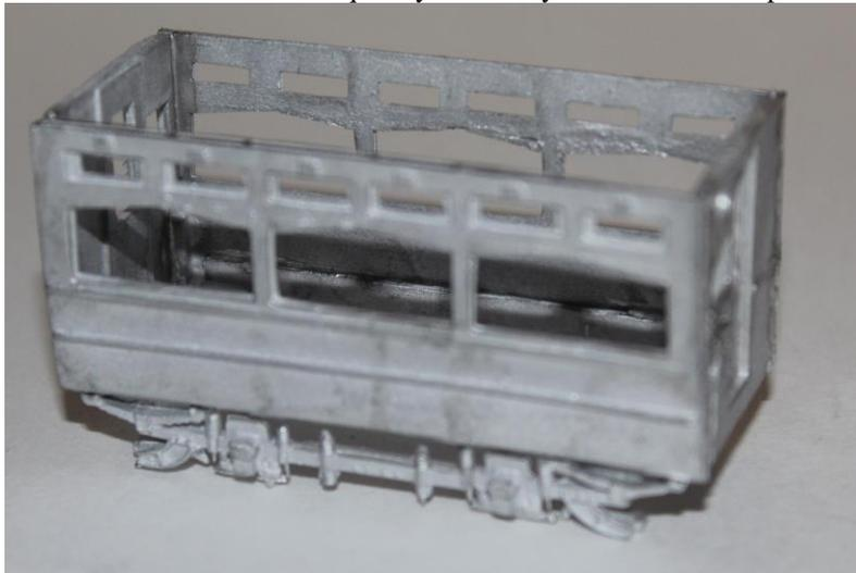
3. With model inverted, attach platforms to bottom edges of bulkheads; ensuring the lip is within the body and not on the platform.
