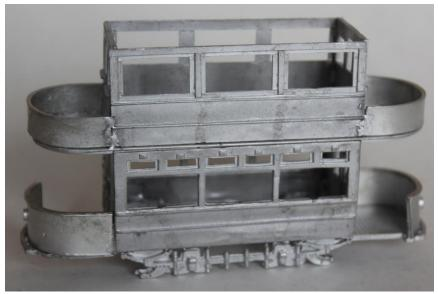
8. Turn model over and fit the steps, fix the life guards under the front panels and the life trays attached to the front edge of the truck sides so they do not interfere with the mechanism.
