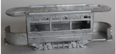
6. Build the upper deck sides & bulkheads on the upper deck floor to form a box.
