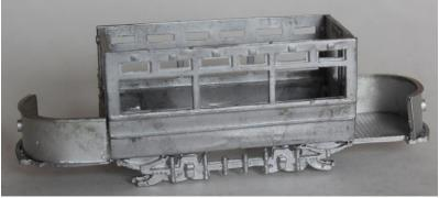
5. Fix the ceiling/upper deck floor piece
