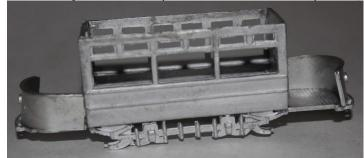
5. Enlarge the stair hole at each end of the upper deck floor to allow the reversed stairs to fit.
