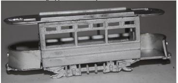
7. Build the upper deck sides & bulkheads on the upper deck floor to form a box.
