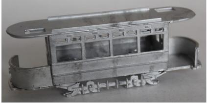
7. Build the upper deck sides & bulkheads on the upper deck floor to form a box.
