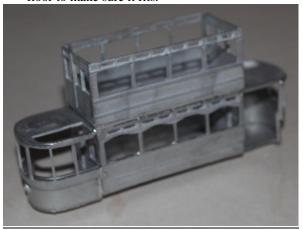
7. Carefully bend the upper vestibule to shape and fit flush to edge of floor. You may need to trim the upper or lower edges of the vestibule to get the height right.
