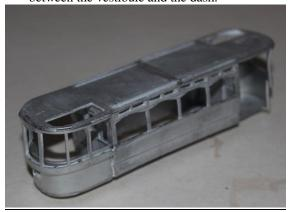
6. Fix upper bulk heads to upper sides squarely and marry the two subassemblies on the upper deck floor to make sure it fits.
