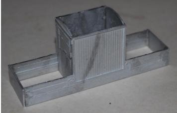
3. With model inverted, attach platforms to bottom edges of outer body ends; flush to the edge.
