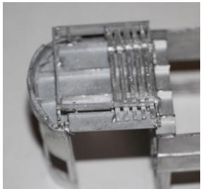
6. Trim the floor to size as required, then fit at the appropriate height to suit the bogies. The bogie mounting points are marked by the dimples in the floor, drill these out if required.
