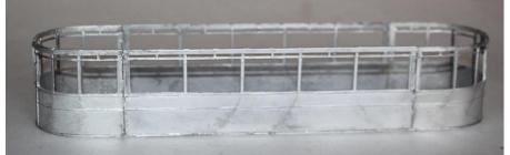
10. If required, fit the additional window frames and destination letter box to the top of the middle vestibule window.
