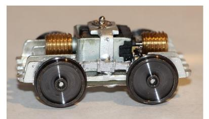
17. If modelling the later style with EMB bogies, fit the bogie ends to the bogie, and the bogie sides to the ends. Fit the track brakes below and behind the middle of the bogie sides. Fit the bogie top bars if required
