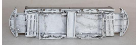
13. Fit a controller and handbrake to each platform. The controller goes just to the left of centre, the handbrake fits in the hole in the platform.
