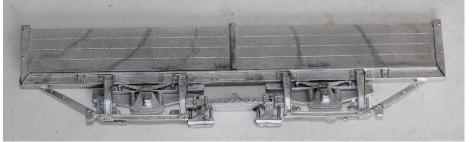
3. Attach the relevant boxes and shelves to the two wagon ends. Make up handrails from wire and fit to wagon ends.
