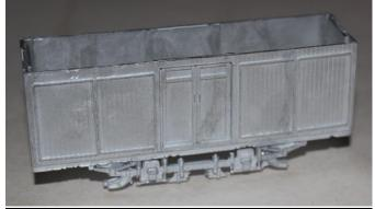
3. Trim the rear outer edges of the platforms to allow them to fit, then fix in place so that the body is flush against the rearmost ridge on the platform.
