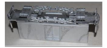
8. Fit the roof and the trolley plank.
