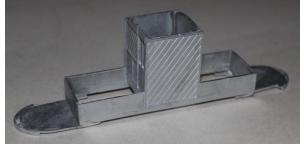
4. Carefully bend the dash panels to fit the curve of the platform, trim to length and fit to platform.
