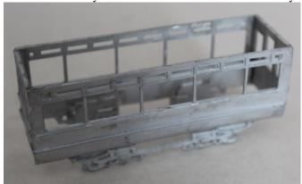
3. Fit the platforms. These should be central, the bulkhead front fitting up to the last floor rib. You will probably need to trim the sides of the platform to get it to fit between the truck sides. If fitting a BEC or ABS truck, you will need to shorten the back end of the platform by 5 mm and extend the depth of the slots to take the mechanism.
