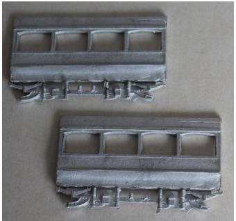
2. Fix bulk heads to sides squarely and marry subassemblies to produce a box effect.
