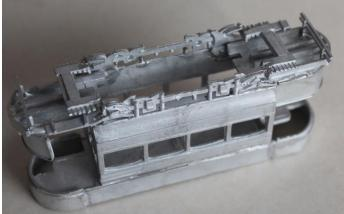
8. Fit the stairs. Note, the stair bases include resistance boxes, but to be more accurate, you can remove these and instead fit the single taller resistance box under the stairs at one end.
