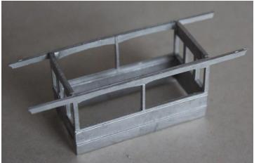
2. Attach truck sides to body sides ensuring exact centrality. You will need to trim the upper section of the truck side to make it fit. In addition, if fitting a BEC or ABS motor, you will need to reduce the length of the motor assembly to make it fit inside the body.
