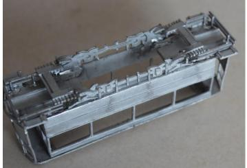
8. Fit the clerestory sides so that they fit just inside the roof. Then fit the clerestory ends.
