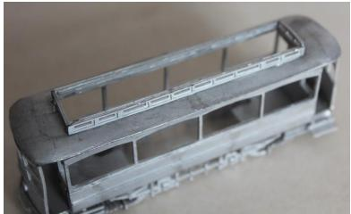
9. Fit the upper roof centrally to the top, and the trolley plank centrally to that.10. Fit the trolley mast and make up a trolley pole from wire11. Fit the destination boxes to the ends of the upper roof.
