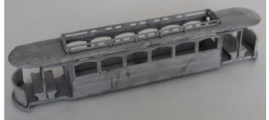
10. Fit the upper roof centrally and fit the trolley plank flush with one end.
