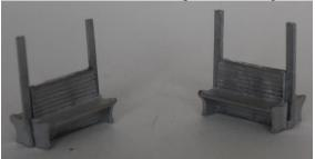
6. Fit the seat assembly to the middle of the platform so that it is flush with the ends of the side extensions.
