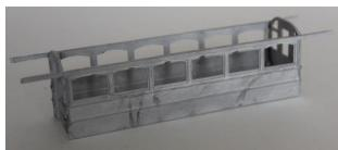
2. If required, fix the bulkhead lights to the top left of the bulkhead.
