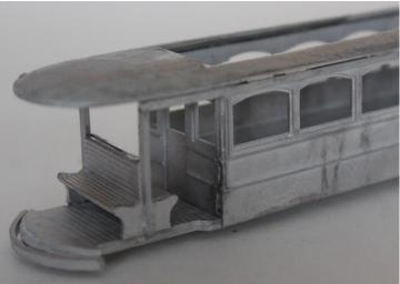
7. Depending on which version of the tram you are making, use the appropriate dash or vestibules. Carefully bend the vestibule or dash panels to fit the curve of the platform and fit to platform.
