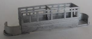
5. Solder the two halves of the ceiling/upper deck floor together and fit.
