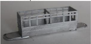
4. Carefully bend the dash panels to fit the curve of the platform, cut to length, and fit to platform.
