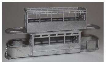
9. Carefully bend the balcony ends to the shape of the floor, cut to length and fit.
