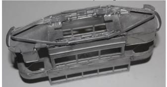
12. Reduce the length of the two roof pieces by 3mm each, then solder the two halves together. Fix the trolley plank to the centre of the roof.
