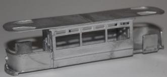
7. Solder the upper deck sides to the upper deck bulkheads to form a box shape.
