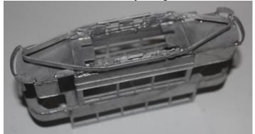
11. Solder the two halves of the roof together. Fix the trolley plank to the centre of the roof. Do not fit the roof until you have painted the interior and glazed the upper deck.
