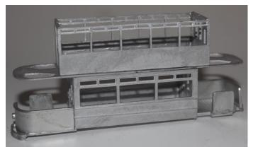
8. Carefully bend the balcony ends to the shape of the floor, cut to length and fit.
