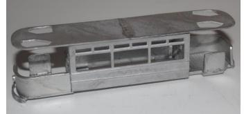
6. Solder the upper deck sides to the upper deck bulkheads to form a box shape.
