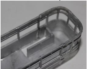
12. Fix one of the upper tall bulkheads at right angles to the upper wide tall bulkhead. Fit over the other stair hole — with the end of the wide section in line with the end of the stair hole and the narrow bulkhead crossing the hole. Fit the other narrow bulkhead 5mm from the stair hole. Do not fit this assembly to the lower deck until you have painted and glazed the lower deck.
