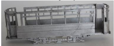
8. Fit the entrance door bulkhead 2 (the widest one) to the side. Fit a platform door between the ridges on the entrance vestibules. Fit the wide door top above the door. Fit the wide doorway filler flush with the outer edge of the vestibule and the side.
