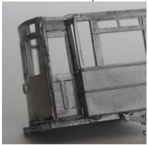
7. Solder the two subassemblies together to produce a box.
