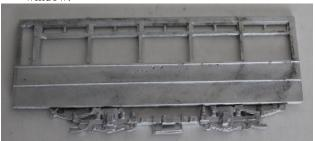
4. Fix the side to the platform (you will need to remove the tab on the left of the platform and cut back the mount on the truck side to get a good fit). Repeat for the other side.
