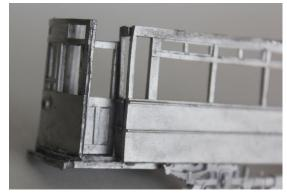
6. Fit the narrow door top above the door. Fit the narrow doorway filler flush with the outer edge of the vestibule and the side. Repeat for the other side.
