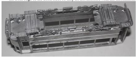
10. Fit the upper sides centrally to the upper floor / ceiling. Carefully bend the upper vestibules to match the shape of the floor end and fit in place (they may require trimming a little).
