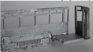
5. Fit the lower exit door bulkhead 2 (the one with only 1 side to the window) to the edge of the side. Fix a platform door behind the 2 small bulkheads. Repeat for the other side.
