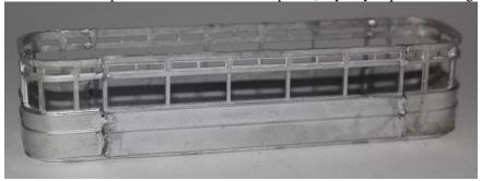
11. Fix the upper low bulkheads together at right angles and fit round the stair hole at one end (this is the end that will have the U shaped / double curved seat fitted once it has been painted.
