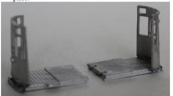
2. Fit the lower exit door bulkhead 1 (the solid bar) to the nearside of the vestibule and the lower entrance bulkhead 1 (the narrow one with 2 sides) to the offside of the vestibule.
