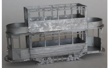
10. Turn model over and fit the steps, life guards under the front platform and the life trays attached to the front edge of the truck sides so they do not interfere with the mechanism.
