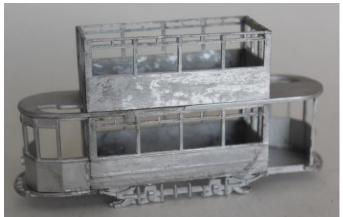
9. Carefully curve the balcony ends to a smooth curve and fit flush to edge of upper deck sides and is approximately 3mm shorter than the floor. You will need to trim the panel to the correct length.
