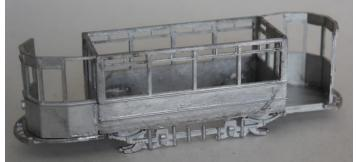
6. Fix the two halves of the ceiling/floor together and fit to the lower deck.
