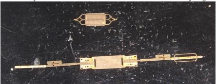
Carefully bend the side thickeners (these are the parts shown by the arrows) with the etched groove on the outside so that it is flat to the bar. I used a fine pair of pliers to do this.
