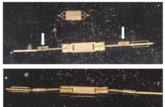
3. Gently bend the seat sides down then the next section up, then the outer piece down. This makes a "pin" at the bottom, which fits into the slot in the toastrack floor.
