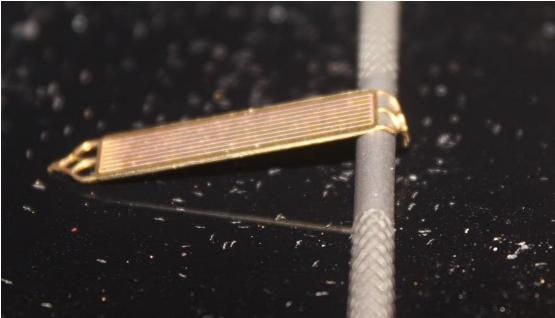
5. Carefully bend the pins at the outer ends of the seat backs outwards so that they can fit in the seat uprights.
