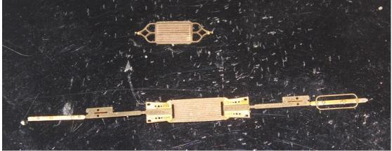
2. Carefully bend the side thickeners (these are the parts shown by the arrows) with the etched groove on the outside so that it is flat to the bar. I used a fine pair of pliers to do this.
