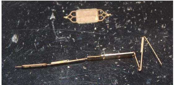
4. Carefully bend the ends of the seat backs into a curve – I used the shaft of a needle file to make the bend.
