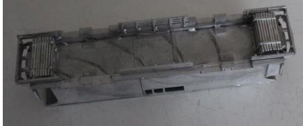
16. Drill a hole in the middle of the roof and fit the trolley mast.
