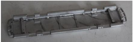
Carefully bend the dash panels to fit the curve of the floor and fit flush to the ends of the floor.
