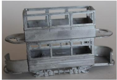
7. Carefully bend the balcony end panels to the shape of the floor, trim to the correct length & fit.
