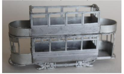
9. Turn model over and fit the life guards under the front panels and the life trays attached to the front edge of the truck sides so they do not interfere with the mechanism.
