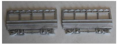
2. Fix bulkheads to sides squarely and marry subassemblies to produce a box effect. You will need to trim the lower edges of the bulkheads or thin the sides to make them fit together.
