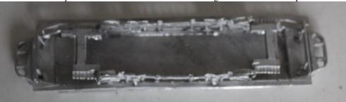
7. Carefully bend the dash panels to fit the end of the floor and fit to floor.
