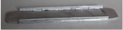
2. Fit the truck sides under the step extensions with the upper extension sections in the gaps.
