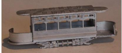
6. Attach upper deck sides to the floor. Carefully bend the upper deck end to shape, cut to length and fit.
