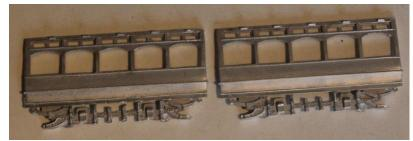
2. Fix bulk heads to sides squarely and marry subassemblies to produce a box effect.
