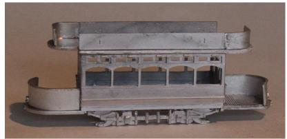
Turn model over and fit the steps and the life trays attached to the front edge of the truck sides so they do not interfere with the mechanism. Fit the lifeguards.
