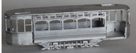
7. Fix upper bulkheads to upper sides and marry subassemblies to produce a box effect.
