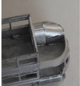
12. For the closed end, fit the stair cover arch, then the short slatted stair cover against the side of the tram. Then cut and fit the stair partition and the curved stair cover top.
