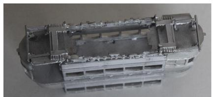
11. Fit the stair covers – open at one end and closed at the other. For the closed end, either fit the curved slatted stair cover or one of the stair cover arches and bend the slatted stair cover to fit. This goes against the upper bulkhead with the arch against the bulkhead. Then fit the stair partition in the gap between the slatted cover and the balcony end – trimming its length and height to fit. Then fit the curved stair cover top and fill as required.
