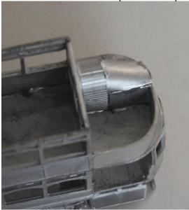
12. For the closed end, fit the stair cover arch, then the short slatted stair cover against the side of the tram. Then cut and fit the stair partition and the curved stair cover top.
