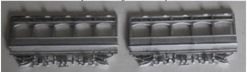
2. Fix bulk heads to sides squarely and marry subassemblies to produce a box effect.
