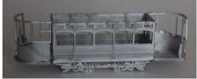
6. Fix the ceiling/upper deck floor piece
