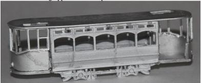
7. Fix upper bulkheads to upper sides and marry subassemblies to produce a box effect.
