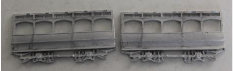
2. Fix bulk heads to sides squarely and marry subassemblies to produce a box effect.
