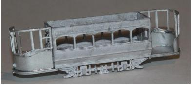
6. Turn model over and fit the steps and the life trays attached to the front edge of the truck sides so they do not interfere with the mechanism. Fit the front, side and step lifeguards.
