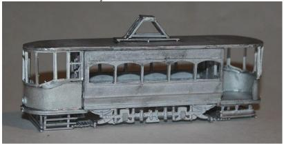
10. Fit the roof side panels and end panels to form a box.
