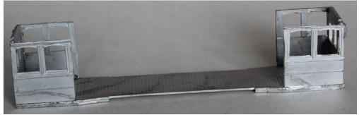
4. Fit the side into the gap between the end assemblies with the bottom in the cut out in the floor.
