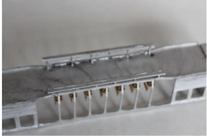
10. Fix the two halves of the roof together. Fit the two halves of the trolley plank together.
