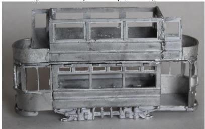
12. Turn model over and fit the steps and the life trays attached to the front edge of the truck sides so they do not interfere with the mechanism. Fit the side and front lifeguards.
