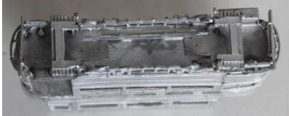
13. Fit the trolley plank to the centre of the roof.
