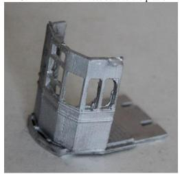
4. File the back edge of the driver vestibule and the edge of the additional window so that the platform fits neatly against the bulkhead.
