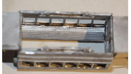
8. Fit the upper seat ends and the upper seat base. Fit the upper deck seats to the upper seat base flush to the outer edge. Fix the upper deck seat backs back to back, then fit to the middle of the seats.
