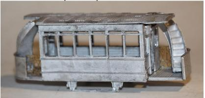
10. Fit the steps to the edges of the platforms. Fit the rear coupler to the lower edge of the rear platform.
