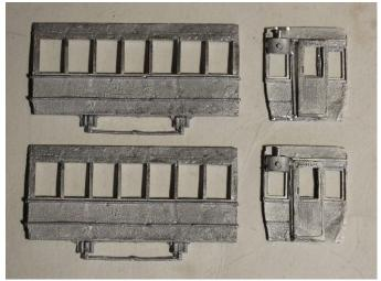
3. Fix bulk heads to sides squarely and marry subassemblies to produce a box effect.
