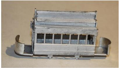
9. Fit the upper floor ends flush to the offside edge of the upper floor.
