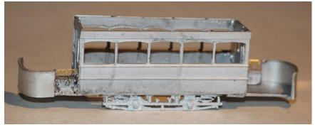
7. On a flat surface, solder the two halves of the upper floor together then fit centrally to the body.
