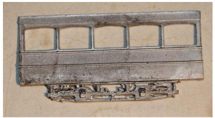
2. Produce the lower saloon box of 2 lower sides and 2 bulk heads by assembly on a flat surface in the upside-down position
